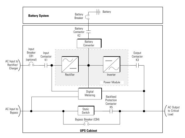
**NOTE** On an UPS configured as an Input Output Module (IOM), the bypass input, static switch, bypass breaker (CB4), and backfeed protection contactor (K5) are not present.
